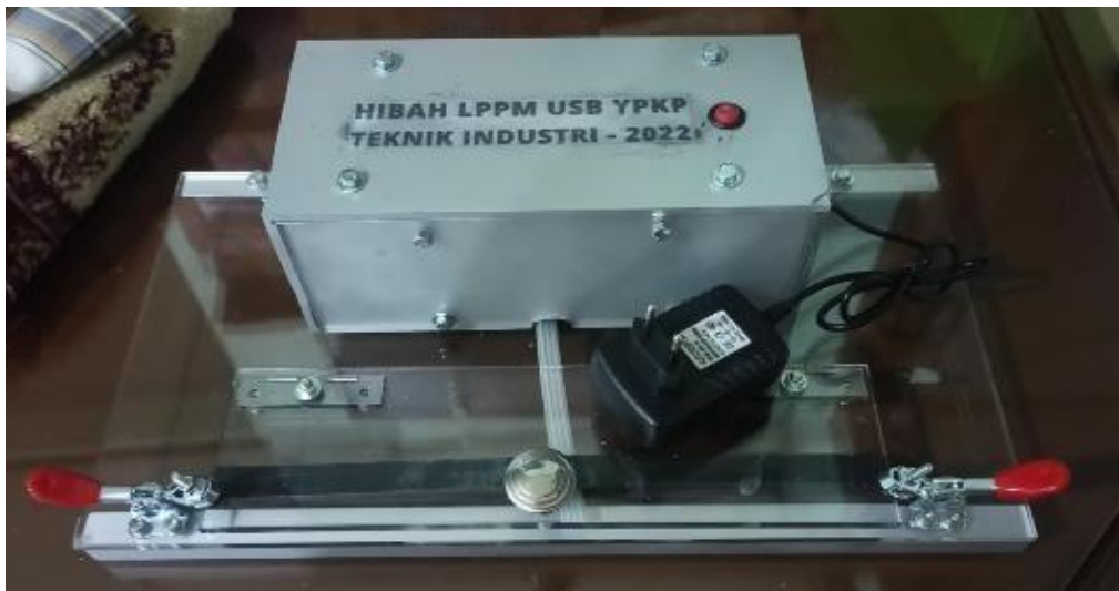
Gambar 5: Prototype Mesin Vacuum Pendamping Sealer Versi 2
