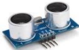
**Gambar 5.** Sensor Ultrasonik (Kularbphetong et al., 2019)
