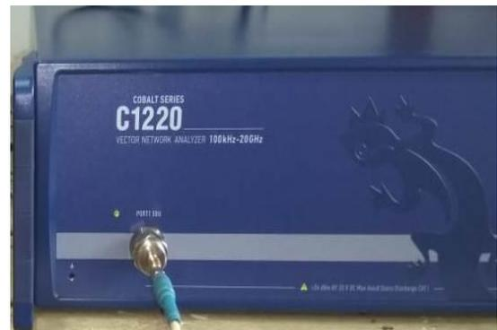
**Gambar 3. 2** Vector Network Analyzer
