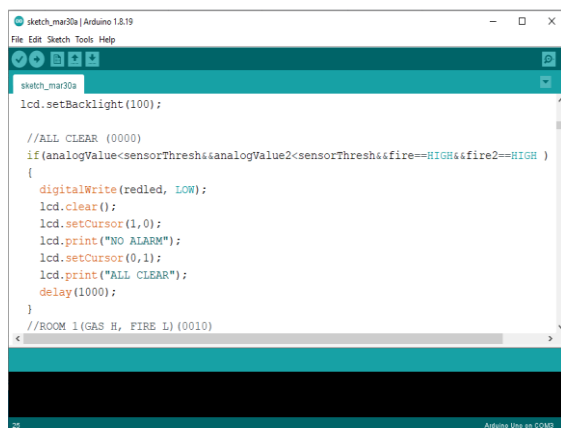
Gambar 12: Program Logika IF Arduino
