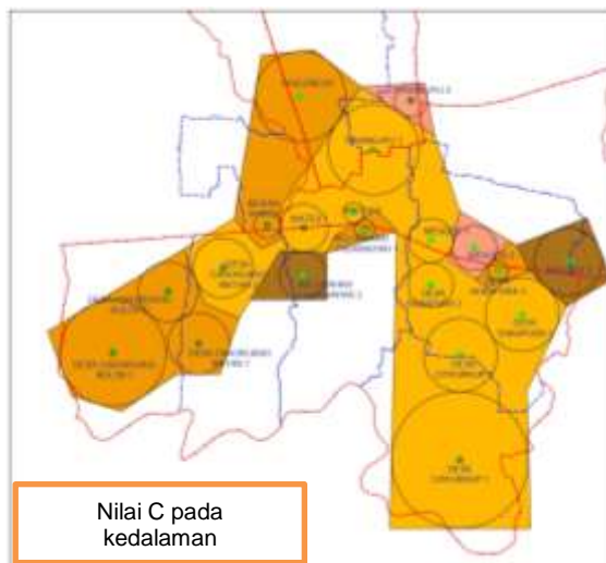
Gambar 26: Peta Konsistensi Tanah Berdasarkan Nilai Undrained Cohesion (C)
