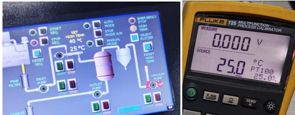
Gambar 7: Pengujian Loop Test Menu Source RTD PT100
